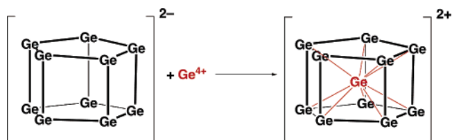
Figure 9. Formation of the centered pentagonal prismatic \text{Ge}_{11}^{2+} (20-5) from pentagonal prismatic \text{Ge}_{10}^{2-} and a central \text{Ge}^{4+} unit (indicated in red).
